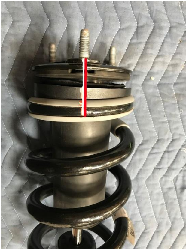
Upper strut mount in OE position
