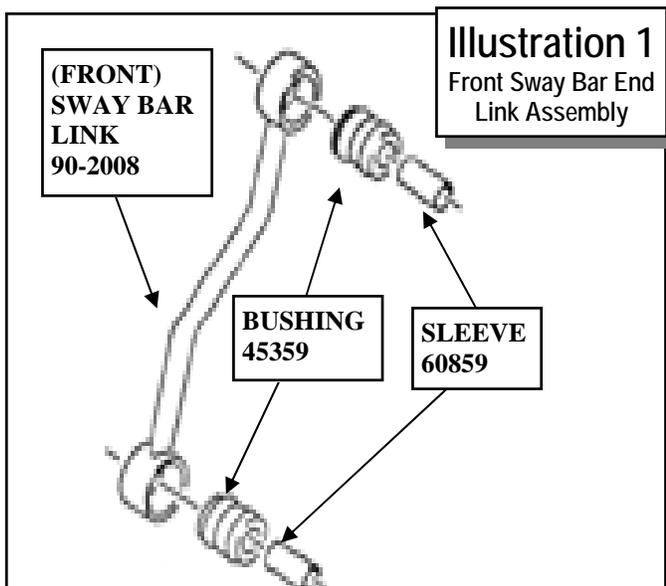
link to the front sway bar using the supplied **12mm X 60mm** bolt and hardware. Torque the **12mm** hardware according to the torque chart on page 10.
