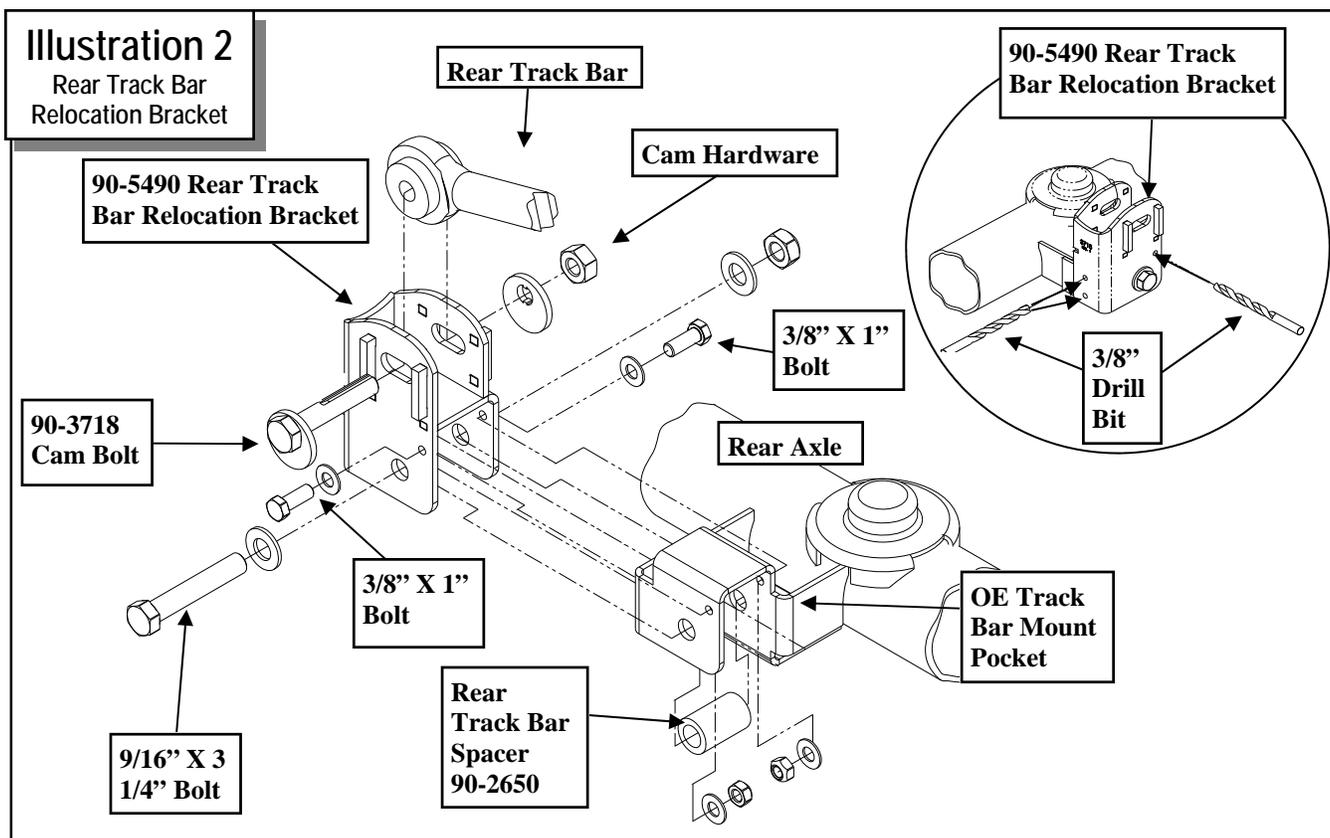
10. Install the rear track bar relocation bracket (90-5490) into the original track bar mounting pocket using the supplied 9/16" X 3 1/4" bolt and supplied spacer (90-2650).
